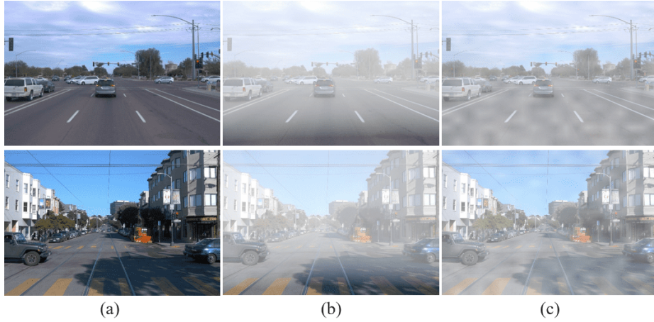
Fig. 2. Synthesized hazy images from WAYMO dataset: (a) Clean images, (b) Synthesized hazy images by the proposed method, and (c) Synthesized hazy images based on random transmission map.
