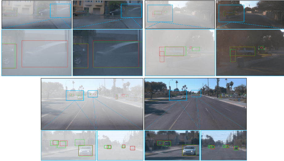
Fig. 6. Application of the EDN-GTM scheme to object detection on WAYMO dataset. In each pair, the left image denotes the hazy image and the right image presents the dehazed image (red box: ground truth, green box: detection).
