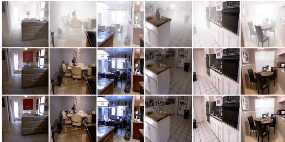
Fig. 4. Visual dehazing results of the EDN-GTM on synthetic hazy dataset D-HAZY (top: hazy images, middle: dehazed images, bottom: ground truth images).
